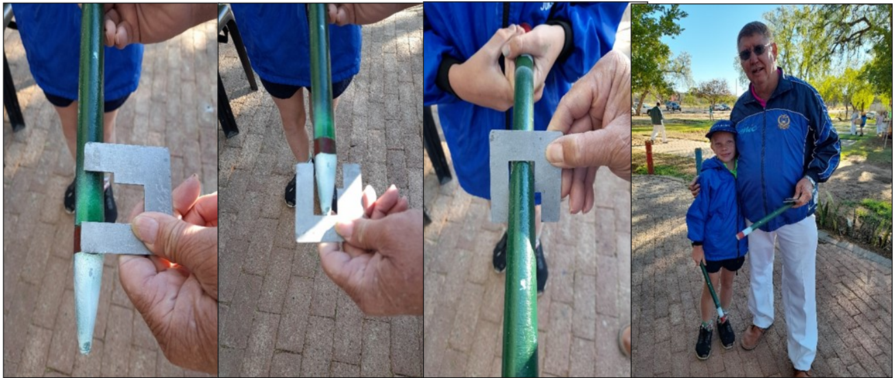
Item 14 Peg Specification Gauge: This junior player came to me asking if his peg is correct, I told him lets find out, and I used the Peg specification gauge to determine if the peg was correct on the first pic. I determined the wind mark to see if it was correct, on pic two I determined the 50mm tapered and on pic three I determined the diameter of the peg.
