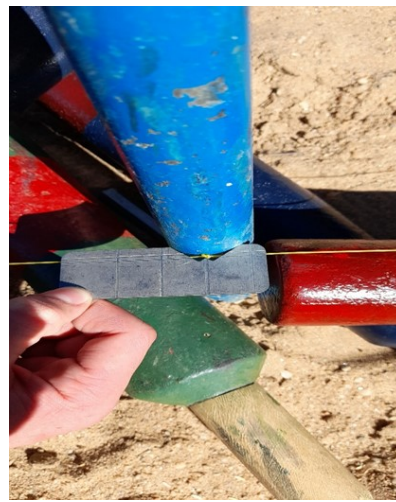
Items 15 and 16: A Large and small Peg position gauge: When the cross string has been drawn across the sandpit, the peg is placed exactly behind the knot, a Peg position gauge is used to determine that the peg was positioned correctly.
