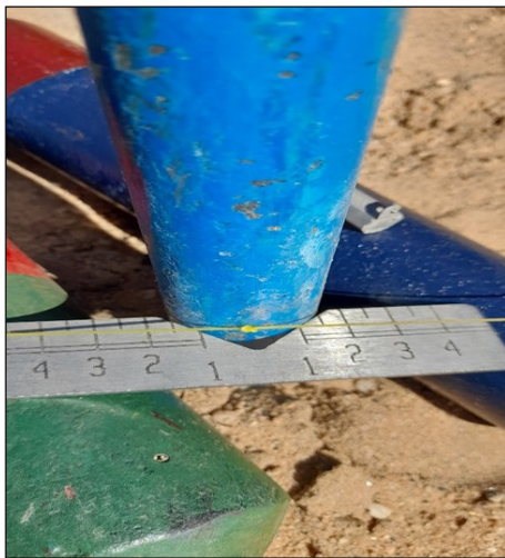
Items 15 and 16: A Large and small Peg position gauge: When the cross string has been drawn across the sandpit, the peg is placed exactly behind the knot, a Peg position gauge is used to determine that the peg was positioned correctly.
