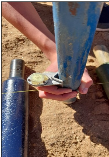
Item 2 Vertical Level: to see that the peg is standing up straight.
