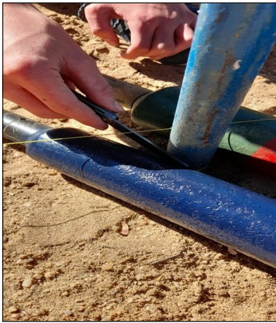
Item 4 Feeler gauge: to measure the distance between the 2 skeys where a caliper will not fit.
